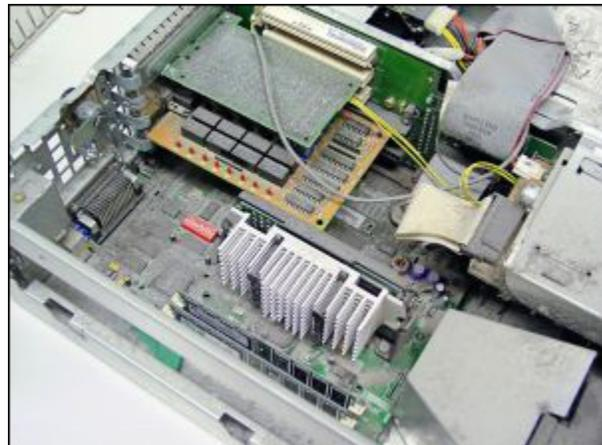
With your can of air, pay special attention to fans on the graphics card, the CPU cooler, and the chipset (if any). If air alone can't clean the parts, you might have to remove them and flush them clean with an aerosol can of electronics cleaner (available at most self-respecting electronics stores).
