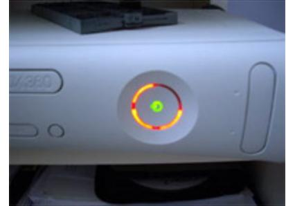
Alternately, you might not even see the Red Ring of Death even when you see red ring segments. For instance, if all four segments glow red, there's an A/V problem; check the seating of the audio-video cable and be sure the switch on the cable is in the correct position for your A/V needs.
